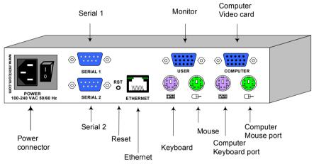
Figure 4 IP Extender ports
